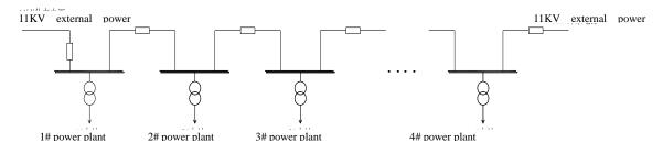
Fig. 3.5 Standby Power Supply Connection Method of the Park
