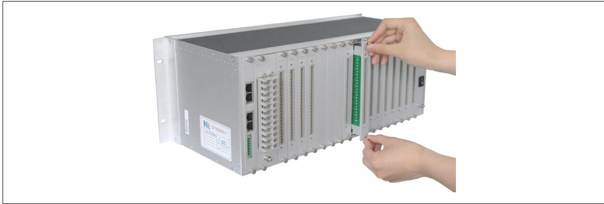
Figure 7.6-2 Demonstration of plugging a board into its corresponding slot
