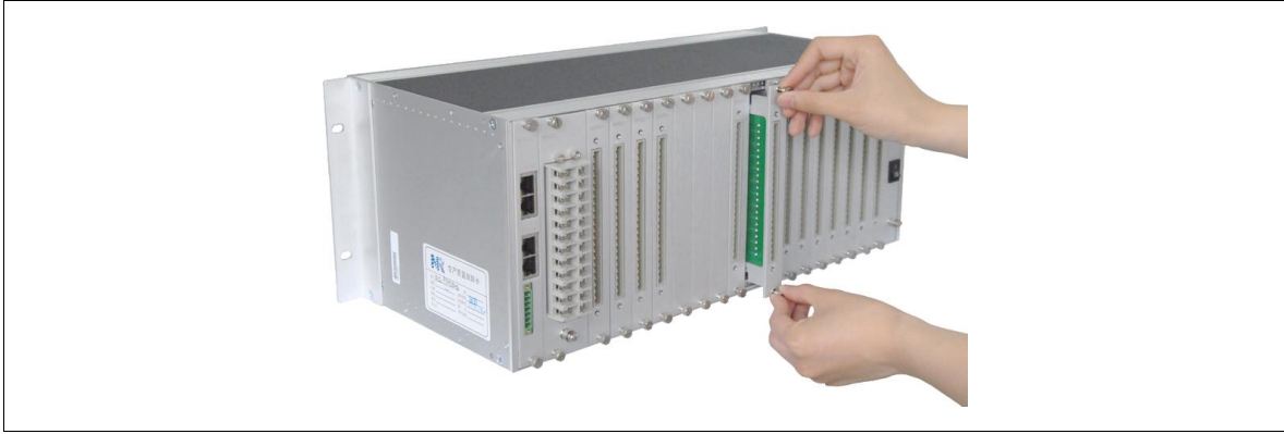
Figure 11.6-3 Demonstration of plugging a board into its corresponding slot
